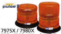
SAE Class I (A & C only) Heavy Duty LED. 5" (7975) and 7" (7980) models, aluminum base, 12-24VDC, 2.8 amps, 11 flash patterns, 3-bolt/ 1" pipe mount, choose color, 2-yr warranty.
