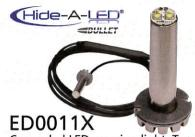
Concealed LED warning light. Two 3-watt LEDs, 16 flash patterns, sync, choose illumination, 1/2" hole mount, self-adhesive, 2", 12-24VDC, IP67, CE, R10, 3-yr warranty.
